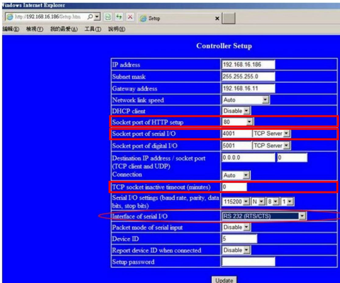
A screenshot of a web browser showing the "Controller Setup" page. The page has a blue background and contains a table of configuration options. Several rows are highlighted with red boxes: "Socket port of HTTP setup", "Socket port of serial I/O", "TCP socket inactive timeout (minutes)", and "Interface of serial I/O".
