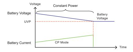
Figure 7 : CP + UVP mode battery discharge test
