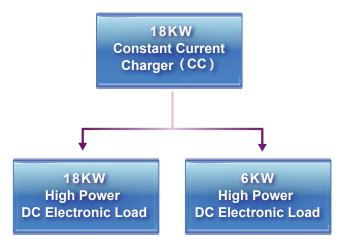
Figure 3 : Single charger connects two loads in parallel
