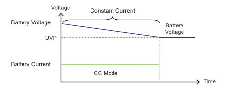
Figure 6 : CC + UVP mode battery discharge test
