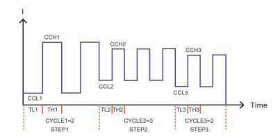
Figure 9: Pulse current discharge / battery discharge test
