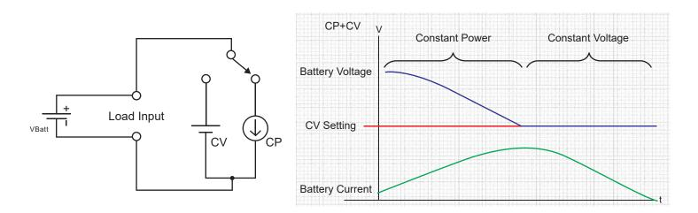
Figure 5: Application of CP+CV operation mode
