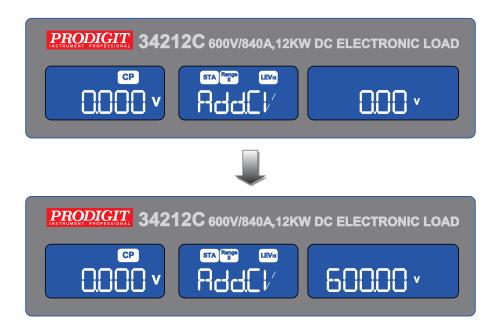
The LCD display shows Add.CV function
