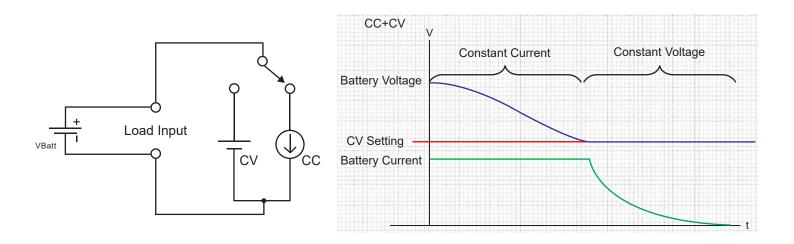
Figure 4 : Application of CC+CV operation mode
