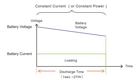
Figure 8 : Setting discharge time battery discharge test
