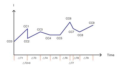
Figure 10: Ramp mode battery discharge test
