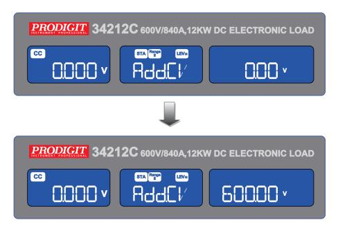
The LCD display shows Add.CV function
