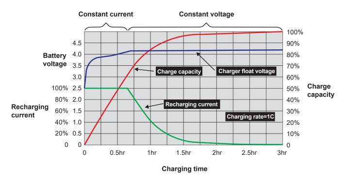
Figure 1: shows a typical charge curve of the battery current, voltage and capacity.
